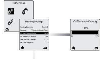
CH Maximum Capacity limits the maximum CH capacity. The appliance capacity can be defined by adjusting this value, 100% means Maximum CH output, 0% means minimum CH output. It is therefore possible to adjust the CH capacity to the installation needs.
