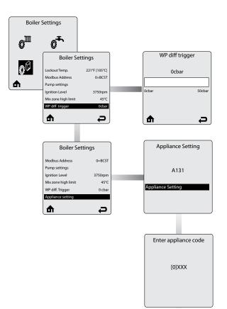
The **WP diff trigger** parameter is the required pressure change when the internal pump is starting. This function allows to detect the correct operation of the appliance internal pump.
