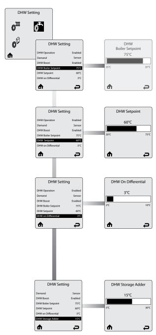
**DHW Boiler Setpoint** is the fixed appliance setpoint temperature during a domestic hot water call when the Thermostat option is chosen in Demand Type.
