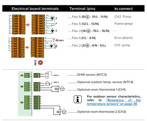
ACVMax interface settings using the Installer menu (Installer code needed, see "Installer Code"):
