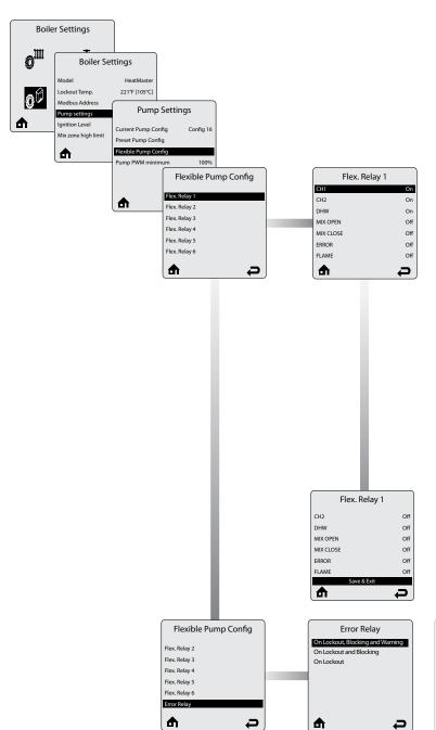
Each relay function has several options. Activation will happen when one of the following options has been chosen: CH1, CH2, DHW, MIX OPEN, MIX CLOSE, ERROR, FLAME.
