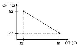
**Outdoor Curve Coldest Day** is the coldest outdoor design temperature of the heating system when an Outdoor Curve option is chosen in Demand Type. This setting is not applicable when a Setpoint option is chosen in Demand Type.
