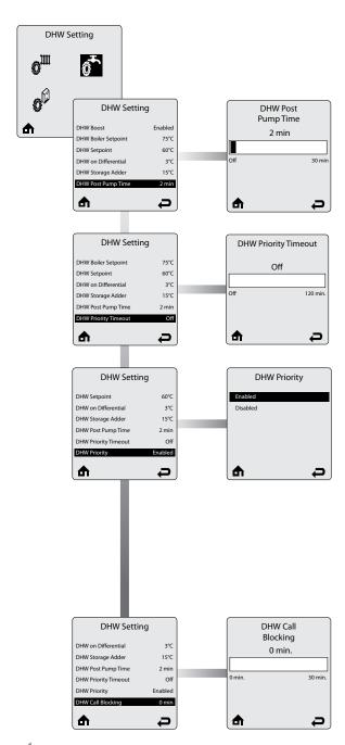
**DHW Post Pump Time** sets how long the domestic hot water circulator will continue to operate at the completion of a domestic hot water call. Any call during the DHW Post Pump Time will be ignored until the post pump has completed. The DHW Post Pump feature allows the heat remaining in the appliance at the completion of a call to be sent to the Indirect Water Heater, which will improve the overall efficiency of the system.
