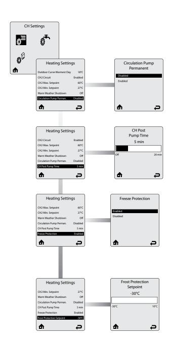
**Circulation Pump Permanent** allows the central heating circulators to be constantly enabled even without a central heating call. A domestic hot water call will cause the circulators to be disabled during the domestic call as long as DHW Priority is enabled.
