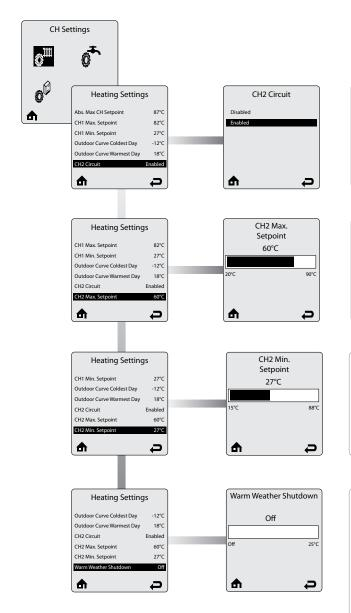
CH2 Circuit allows the CH2 heating call to be enabled and disabled.
