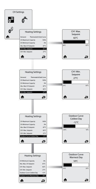
**CH1 Max. Setpoint** is the maximum setpoint for a CH1 heating call when an Outdoor Curve option is chosen in Demand Type. CH1 Maximum Setpoint is the fixed setpoint for a CH1 heating call when a Setpoint option is chosen in Demand Type.
