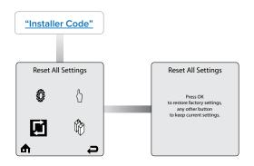
**Reset All Settings** allows the installer to reset all parameters back to the default values (Refer to "Factory settings and reset values" for the default settings).
