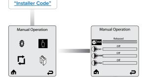
FAN - Touch the OK key while the FAN icon is highlighted to manually fire the burner and power the CH (1) circulator.
