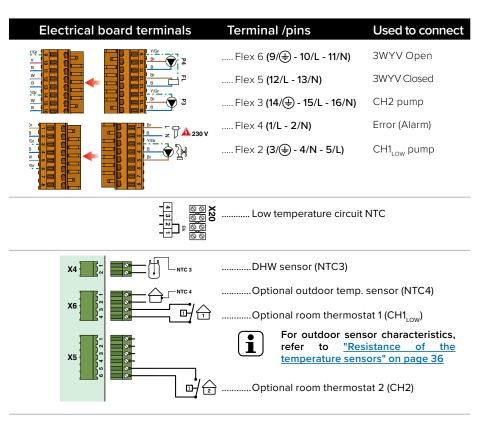
ACVMax interface settings using the Installer menu (Installer code needed, see "Installer Code"):
