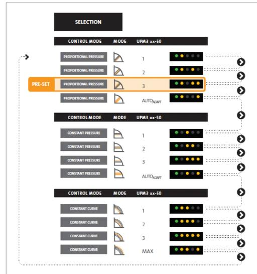
**i** Once the set-up is completed, the pump can be locked to prevent any accidental change. Press the button for more than 10 seconds and all the LED will light (except the red one) and blink for 1 second to indicate that the lock is on. Proceed the same way to unlock.
