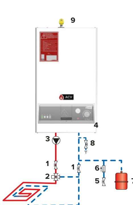
**i** In the case of a floor heating system, make sure that the pump is set to the "Constant pressure" mode.
